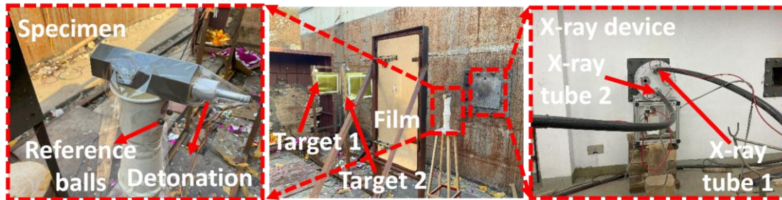
Figure 13. Test setup and schematic.
