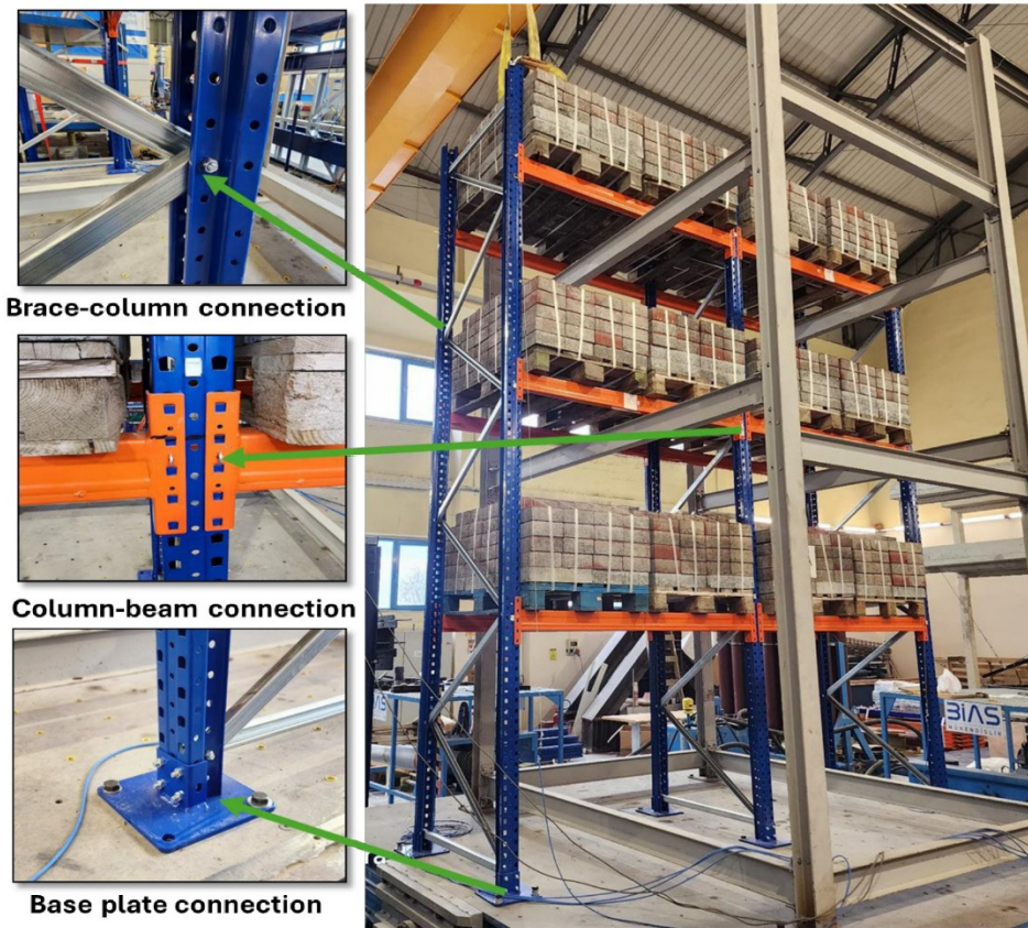
Figure 6 Details of the rack components.
