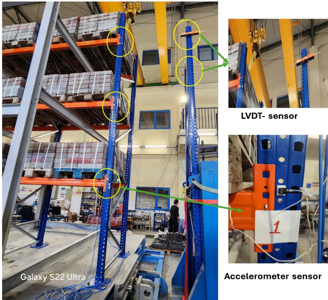
Figure 8 Accelerometer sensor and LVDT placement on the rack structure.
