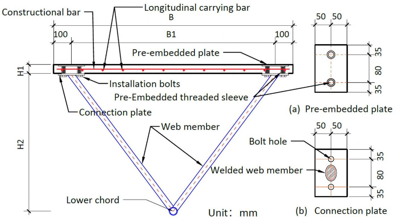
**Figure 4** Construction drawing of install node.
