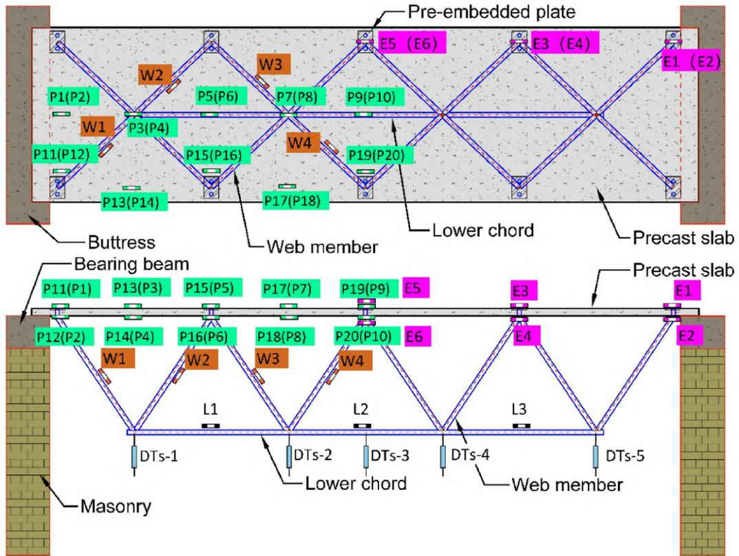
Figure 6 Layout and numbering illustration of strain gauge and displacement meter.
