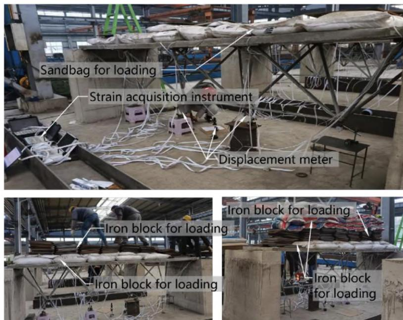
Figure 7 Real scene image of experimental model loading.
