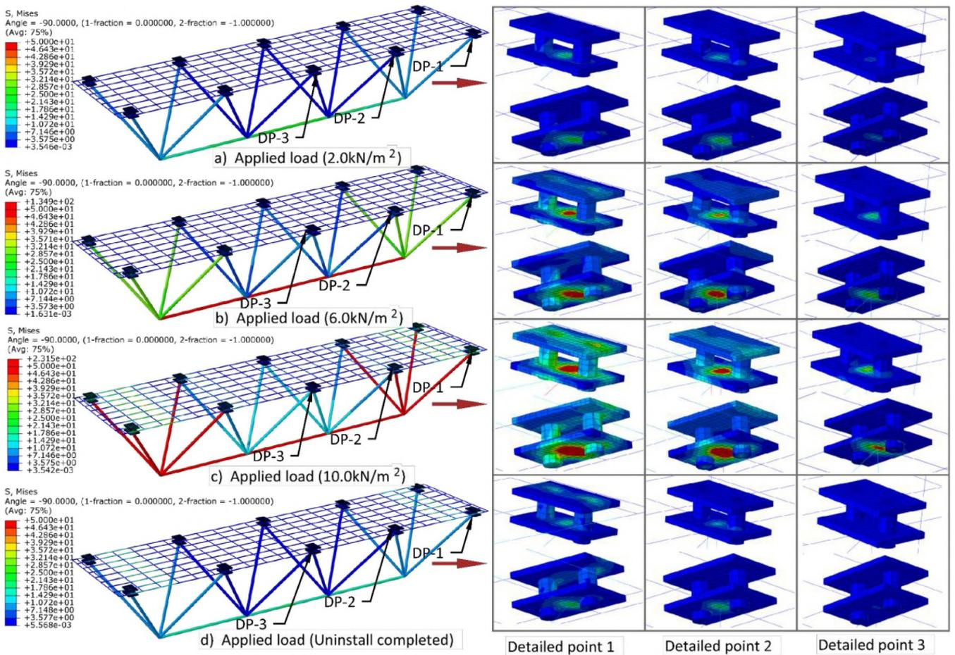
Figure 21 Stress cloud diagram distribution of steel component sections.
