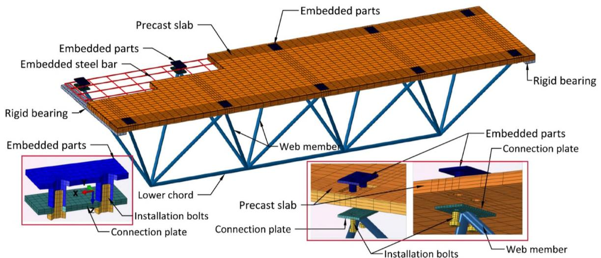
Figure 13 Finite element model schematic diagram.
