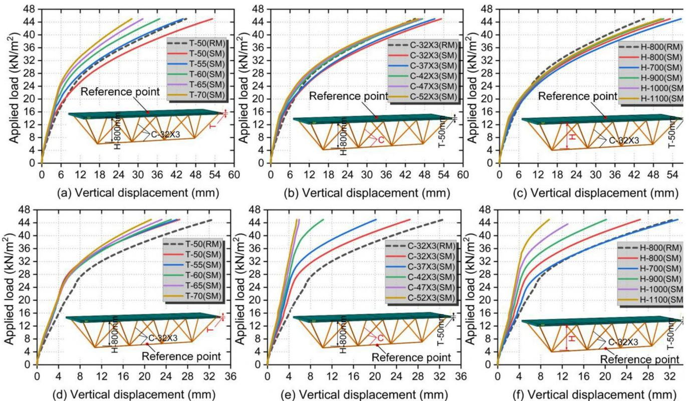
**Figure 22** Vertical load-deflection curve under various parameters.
