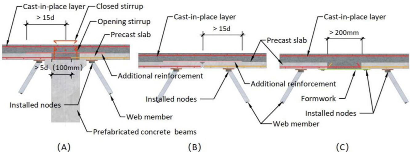
Figure 2 Schematic of assembly joint.
