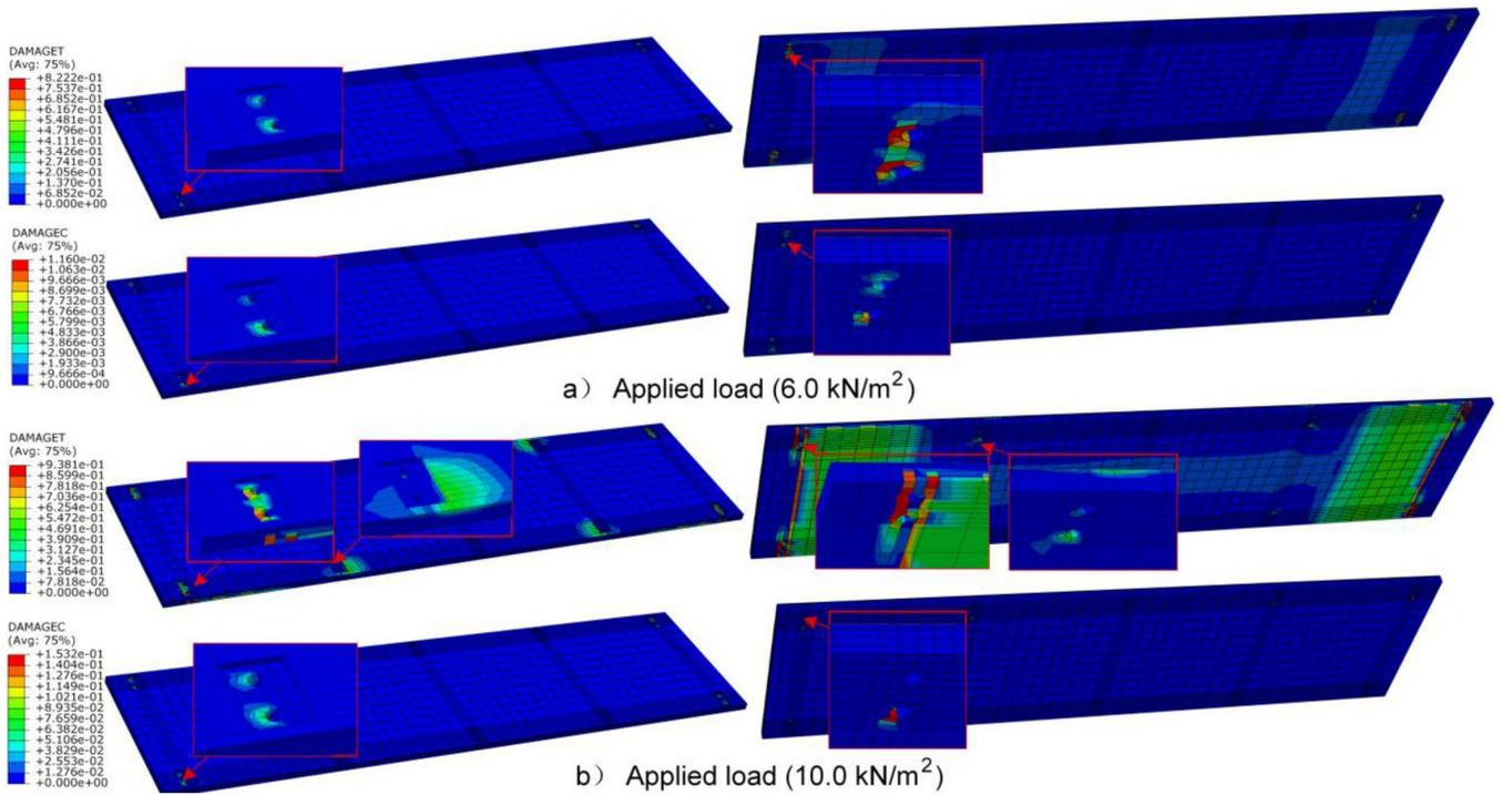
Figure 20 Tensile (DAMAGET) and compressive (DAMAGEC) concrete damage contours.
