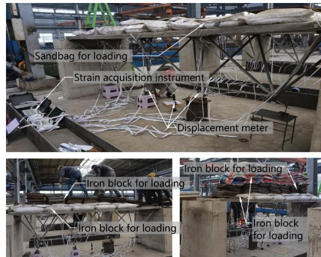
Figure 7 Real scene image of experimental model loading.
