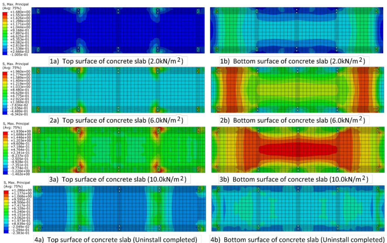
Figure 19 Maximum principal mises distribution of concrete.
