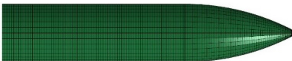
Figure 8 Finite element model of a 20mm projectile.
