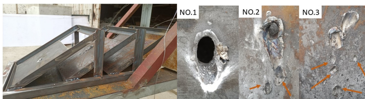
Figure 7. The target and residual penetrator core diagram after penetrating a three-layer target.
