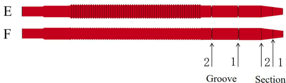
Figure 34. Nosed armor-piercing blocks and weakening grooves of penetrator core.
