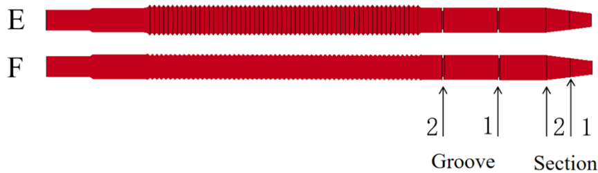
Figure 33. Nosed armor-piercing blocks and weakening grooves of penetrator core.
