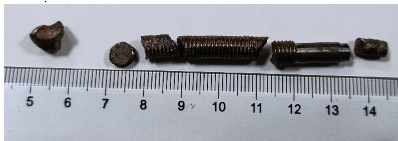
Figure 8. Recovered residual penetrator core through a water tank.
