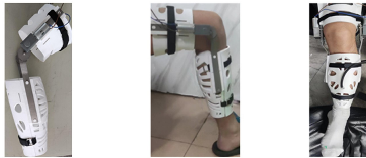
(a) Integral assembly of calf brace (b) Calf circumference 34cm (c) Calf circumference 36cm
