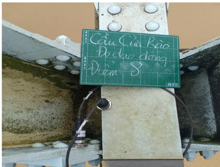
Figure 21 Sensors used for measurements
