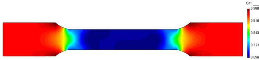
Figure 2 – Contour plot of the component  $G_{11}$  after the damaging phase.
