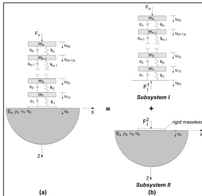
Figure 1 Soil-structure system model and system subdivision.
