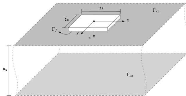
Figure 2 Rigid and massless foundation at the surface of a 3D horizontal layer over bedrock
