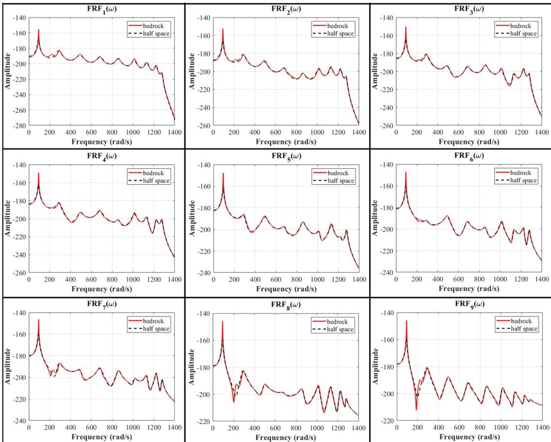
**Figure 6** Structure FRFs with soil influence (System I x System II).
