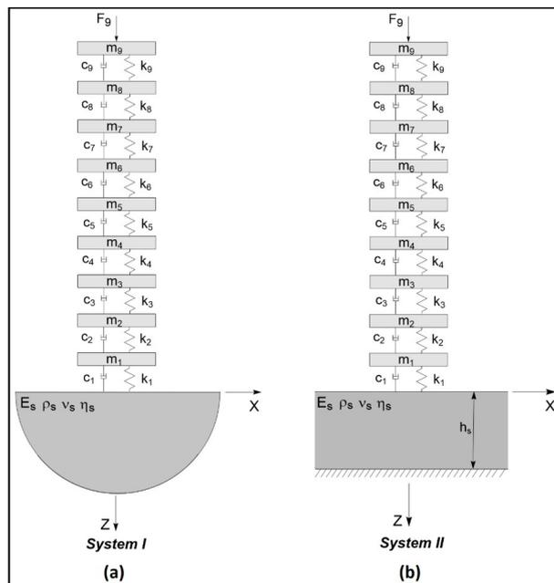
Figure 5 Soil-structure systems with different soil profiles.
