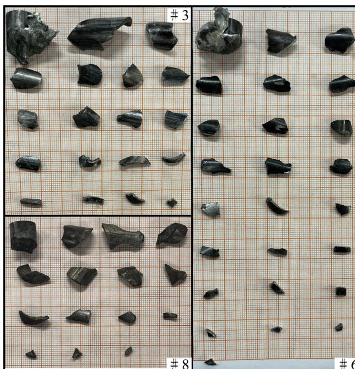
Fig.8 Recovery of fragments of PELE jacket
