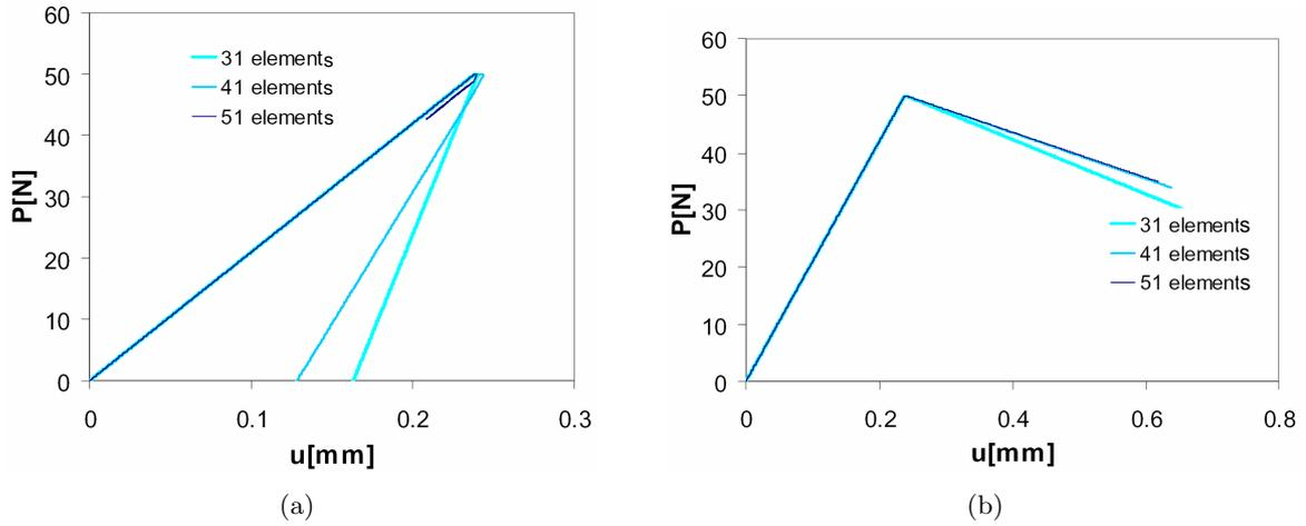
Figure 2: Reaction vs displacement curves for different meshes (a) local model; (b) nonlocal model.
