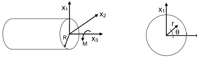
Figure 7: Torsion of thin wires: coordinate systems.
