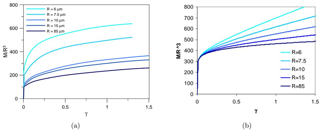
Figure 9: Normalized torque versus normalized twist at  $r = R$  (a) experimental results from [17]; (b) simulation with constant yield stress.
