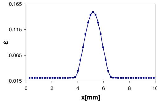
Figure 3: Plastic deformations along the bar, nonlocal model
