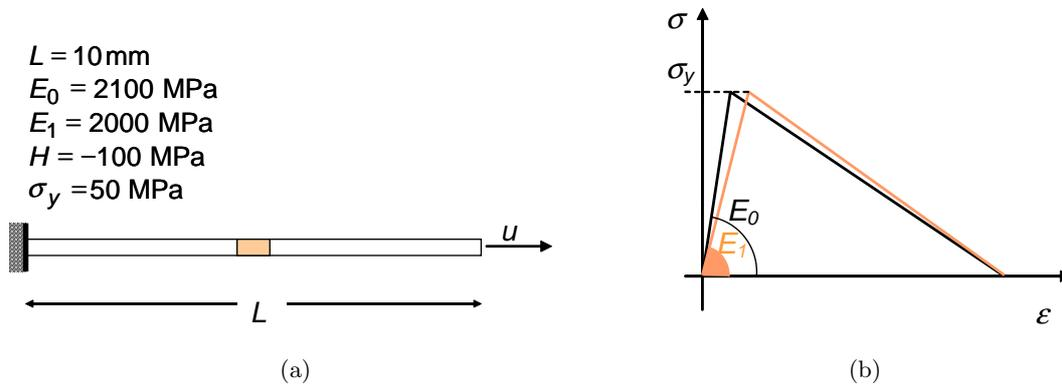
Figure 1: Uniaxial tension test: (a) geometry and material data (b) linear softening law
