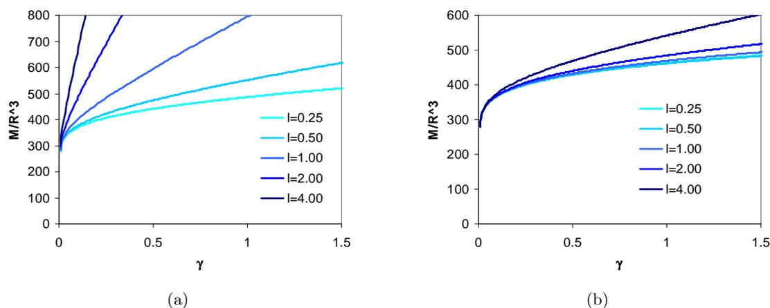
Figure 10: Effect of material length  $\ell$  (a)  $R = 10\mu m$ ; (b)  $R = 85\mu m$
