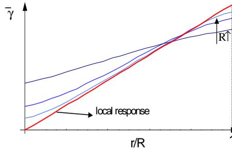
Figure 8: Profile of the nonlocal shear strain for different wire size R
