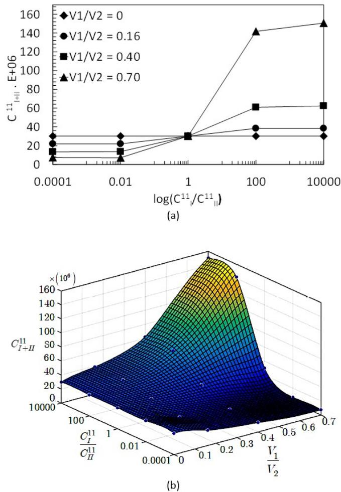
**Figure 13**  $C_{I+II}^{11}$  Value in mesh for different relations of  $C_I^{11}/C_{II}^{11}$  and proportions between volumes.
