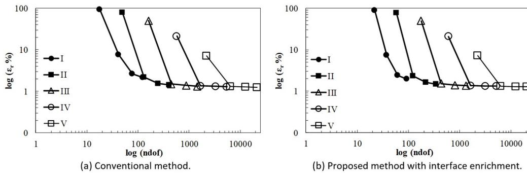
**Figure 8** Relative error,  $\epsilon_r$ , with respect to the ndof for each mesh by adding enrichment functions at different degrees on each mesh for determining the strain energy.
