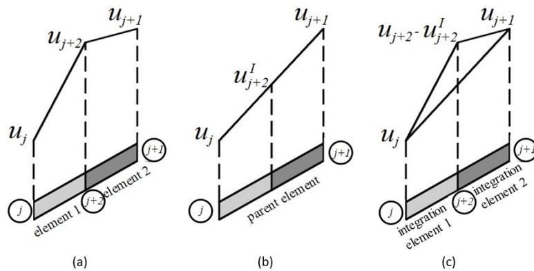
**Figure 2** Approaches in a domain with 2 materials. (a) Conventional FEM interpolation; (b) Interpolation with a non-conforming element; (c) Interpolation using the proposed method with interface enrichment.
