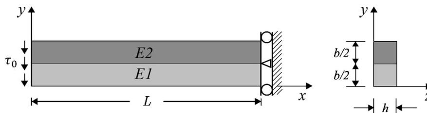
Figure 5. Geometry and loading of the two-material-composed beam subjected to simple bending.
