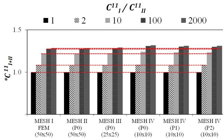
**Figure 12** Normalized  $*C_{I+II}^{11}$  values for different meshes and types of simulations with different  $C_I^{11}/C_{II}^{11}$  relations.
