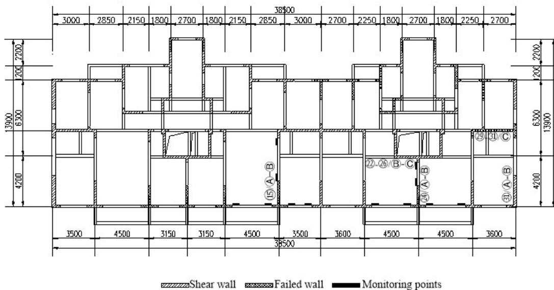
Figure 6 Shear wall structure layout and failure walls
