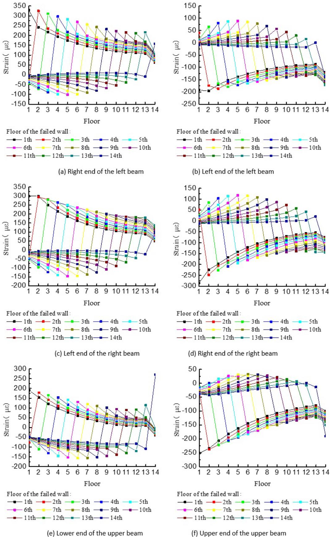
Figure 8 Strains at the ends of adjacent beams when shear wall ⑮/A-B is removed
