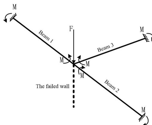
**Figure 2** Stress mechanism of the structure when the edge wall is failed
