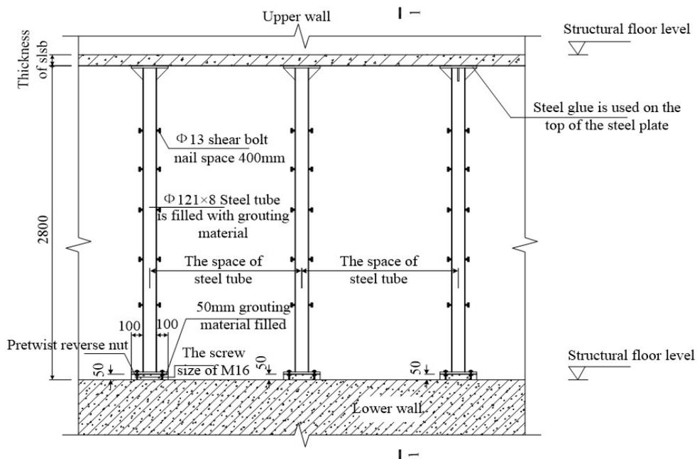
Figure 11 Permanent support facade layout
