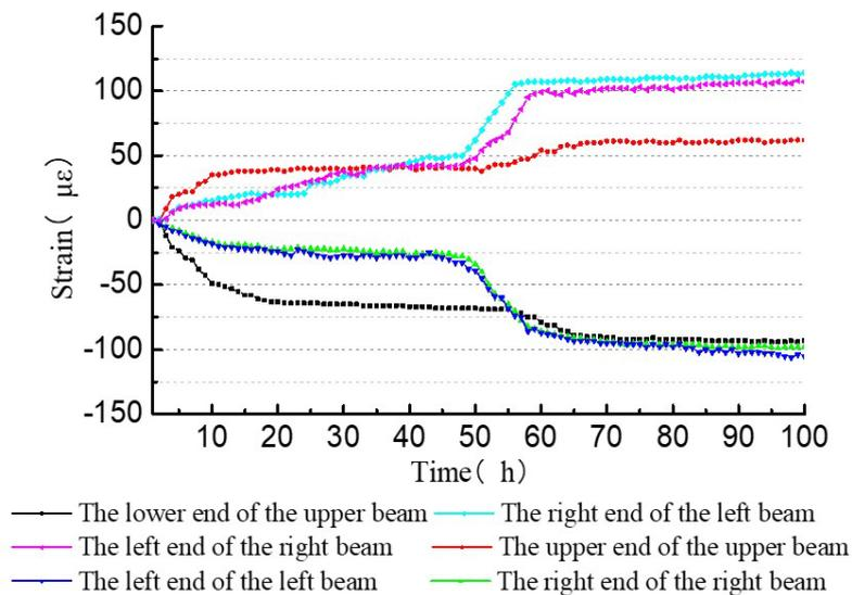
Figure 15 Strains at the ends of adjacent beams when the ⑮/A-B wall is removed on the 6th floor
