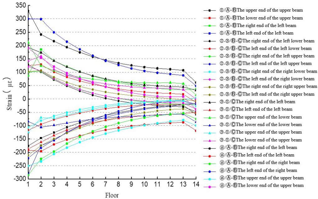
Figure 9 Strains at the ends of adjacent beams when key members are removed on the 1st floor
