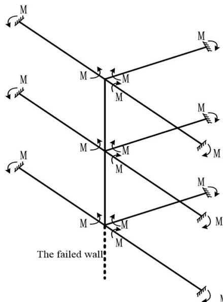
Figure 4 Stress of the substructure when the edge wall is removed
