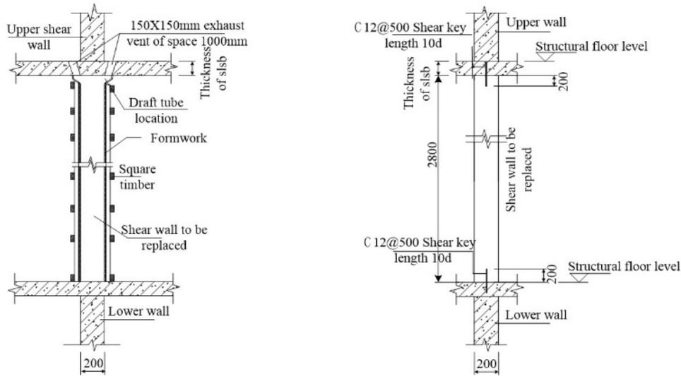
(a) Wall replacement pouring schematic (b) Schematic of replacement connector
