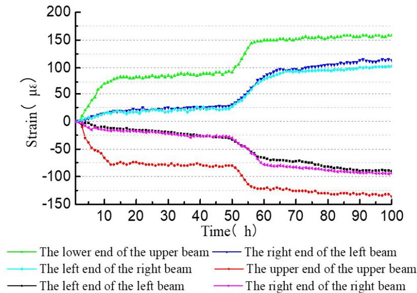
**Figure 16** Strains at the ends of adjacent beams when the ②④/Ⓐ-Ⓑ wall is removed on the 6th floor
