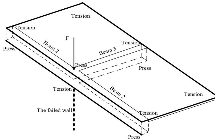
Figure 3 Strains when the edge wall fail
