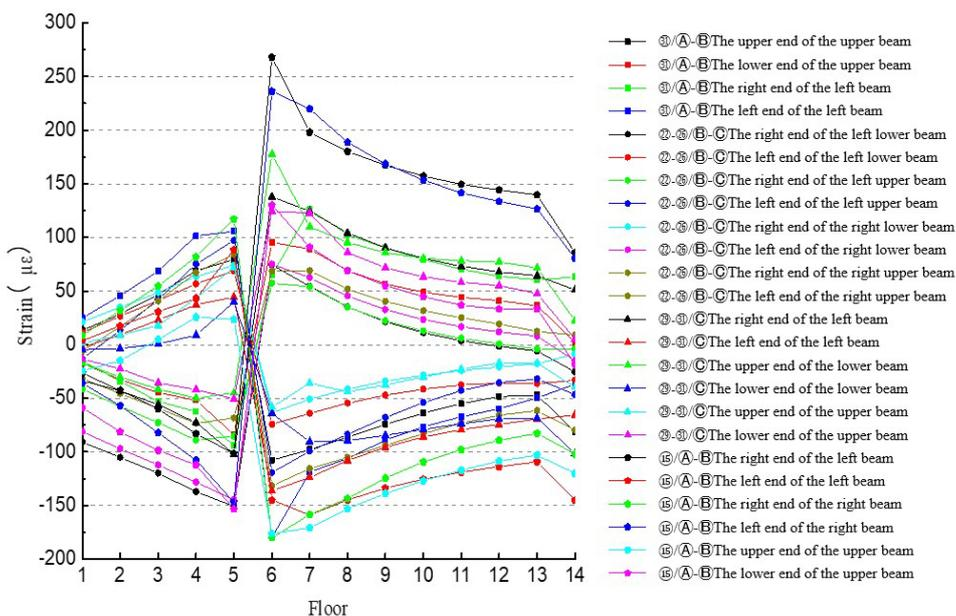
Figure 10 Strains at the ends of adjacent beams when key members are removed on the 6th floor
