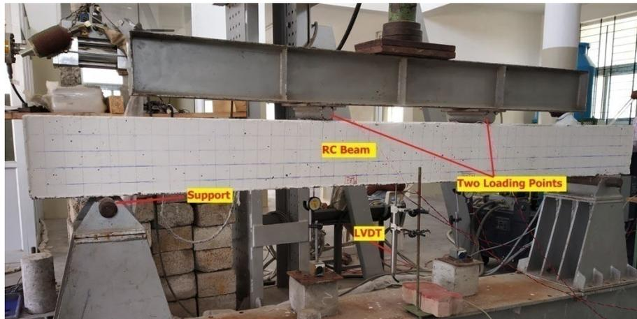
Figure 4 Experimental test set-up of the beams incorporated with PZTs
