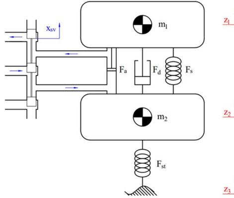
Figure 1: Model of the vehicle dynamics.
