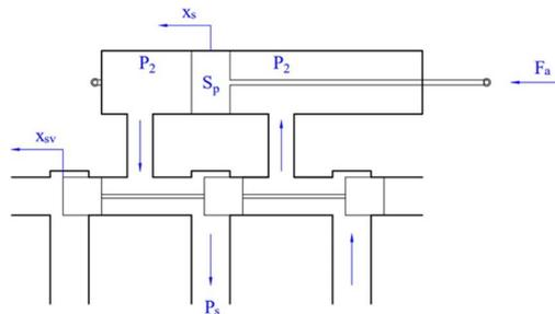
Figure 2: Hydraulic actuator.
