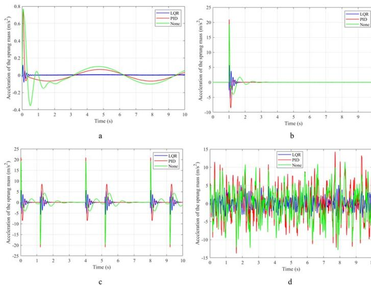
**Figure 6:** Acceleration of the sprung mass (a – Sine wave; b – Step; c – Pulse; d – Random).
