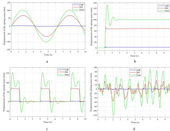
**Figure 5:** Displacement of the sprung mass (a – Sine wave; b – Step; c – Pulse; d – Random).
