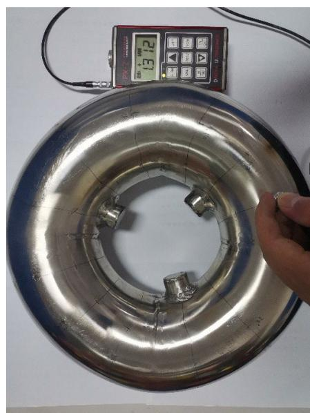
**Figure 5** Thickness measurement.
