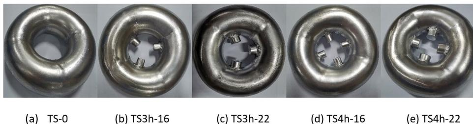
**Figure 3** The test models of toroidal shell with openings; TS represents the toroidal shell, and 3h and 4h represent the openings number of toroidal shell, respectively. 16 and 22 represent the actual hole diameter of toroidal shells.
