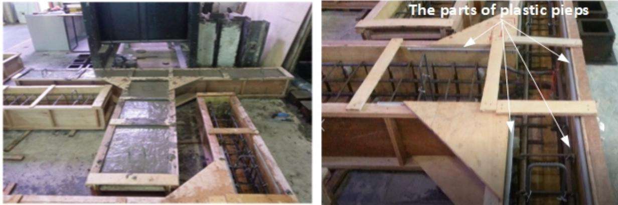
Figure 4: Plastic pipes parts before casting and the casted specimen in the moulds.
