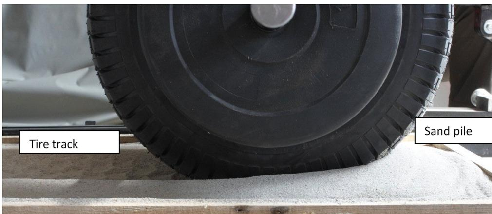
**Figure 14:** The wheel on the experimental stand, after test with  $\alpha_w = 0^\circ$ .
