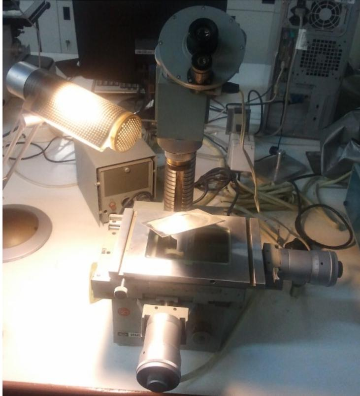
*Figure 11: Callipered microscope used in experiments*
