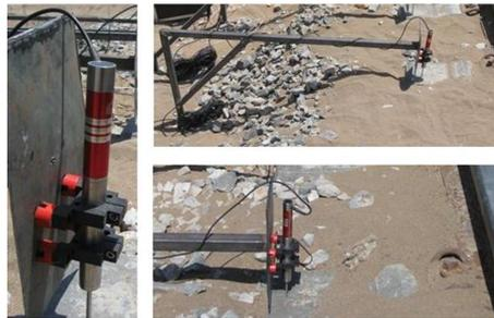
Figure 4 How to put the LVDT devices in tests place, using steel bases
