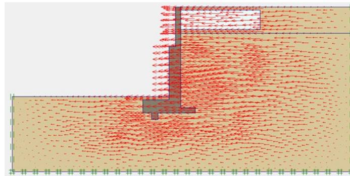
**Figure 11:** Solution 2.b - Combination B. Horizontal displacements. Horizontal maximum 13.54 mm (absolute maximum 14.33 mm).
