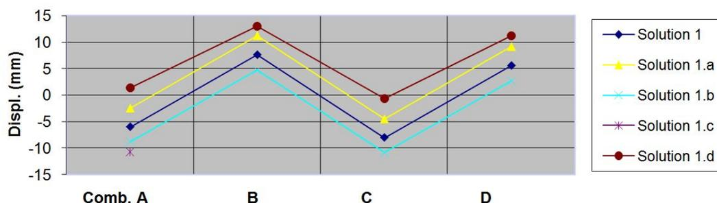
**Figure 6:** Comparison of horizontal displacements in the upper area of the wall obtained with the program Sap 2000. The positive sign would indicate displacement in the direction of the wall rear area (universal coordinate system).
