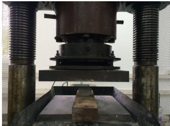
**Figure 14:** *The position of a specimen and loading plates*
