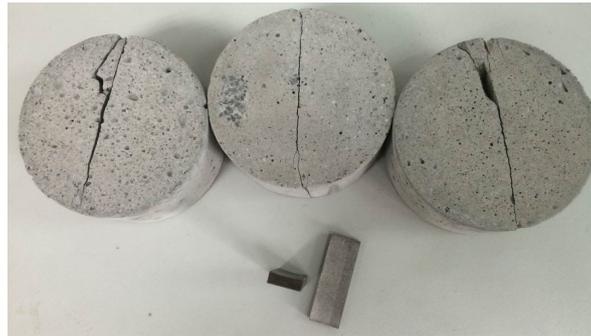
**Figure 4:** The specimen failure pattern and loading strips
