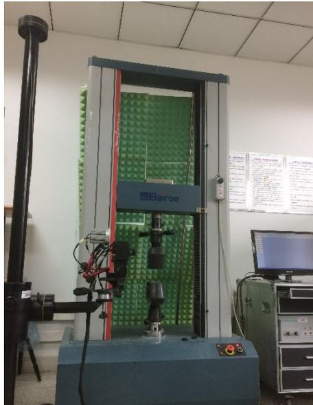
**Figure 2:** WDW-100 double-column microcomputer control electronic testing system
