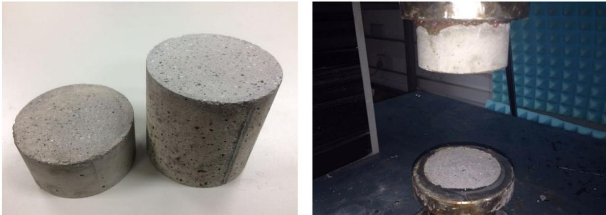
(a) The specimen after treatment of water jet
