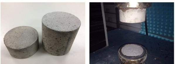
(a) The specimen after treatment of water jet
