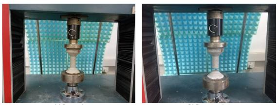
(a) Pre-testing (b) Post-experiment *Figure 11:* The quasi-static direct tensile test of a dumbbell-shaped mortar specimen with the tube
