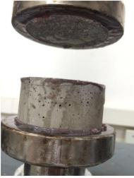
(a) Pre-testing (b) Post-experiment *Figure 7:* The quasi-static direct tensile test of a mortar specimen when the slenderness ratio is 0.5
