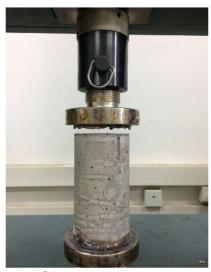
(a) Pre-testing (b) Post-experiment *Figure 5:* Experiment results of a quasi-static direct tensile test of mortar specimen when the slenderness ratio is 2
