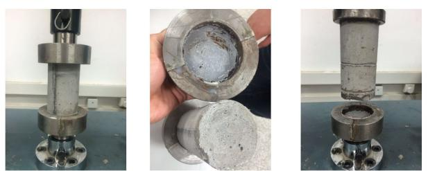
(a) Pre-testing (b) failure fracture (c) notched specimen *Figure 6: The modified direct tensile testing of a mortar specimen*
