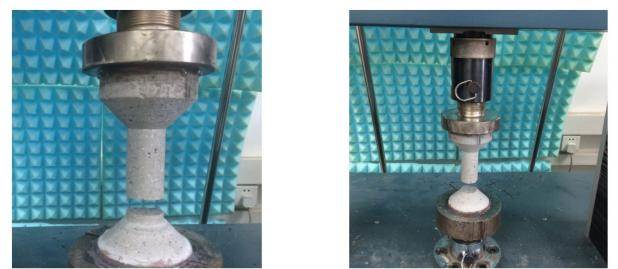
(a) 3.68 MPa (b) 2.97 MPa *Figure 12: Results from quasi-static direct tensile tests of dumbbell-shaped mortar specimens*
