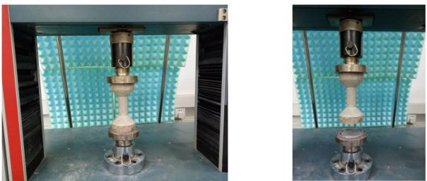
(a) Pre-testing (b) Post-experiment *Figure 10:* The quasi-static direct tensile test of a dumbbell-shaped mortar specimen
