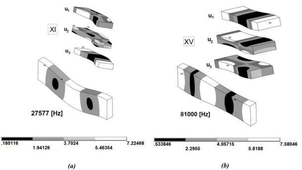
Figure 18: (a) The mode configuration on the curve b (see Figs.9 and 15)(A bending mode around the  $x_2$  axis), (b) The mode configuration on the curve a(see Figs. 9 and 15)(A longitudinal Mode). In both cases it was used the method 2 with  $k=100m^{-1}$  and p=1.
