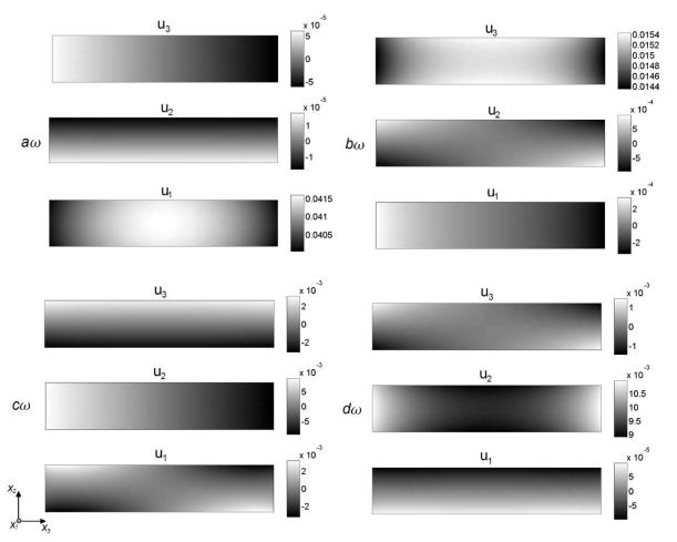
**Figure 11:** The modal displacement for the wave modes linked with the curves a,b,c,d, at the frequency of 50KHz. (see Fig. 9). Here the axis  $x_2$  and  $x_3$  are in the transversal section of the guided waves considering  $x_1$ , in the guide propagation direction. The modal displacements were obtained using the Method 3, described below.
