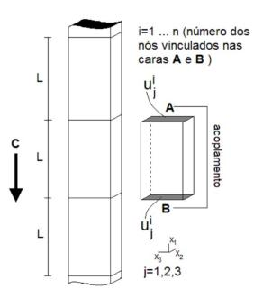
Figure 8: Rectangular stem portion, detail about how the boundary conditions were applied.
