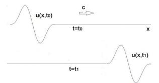
*Figure 2:* One-dimensional wave propagation, without distortion and losses.  $t_0 < t_1$ .
