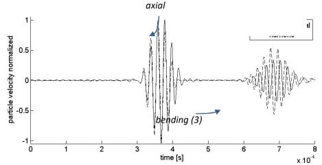
*Figure 24:* Results in terms of the velocity in the dir. 1 due to the longitudinal excitation applied (a tone burst function with a central frequency of 50KHz). Axial and bending wave modes around the axis (3) appear in the plot. The point, where the response is measured, is found at 1.5meter from the excitation applied. Experimental result in continuous line, Numerical result in discontinuous line.
