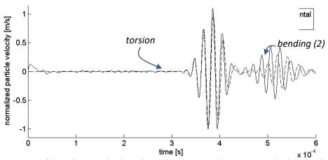
Figure 23: Results in terms of the velocity in the dir 3 due to the transversal excitation applied (a tone burst function with a central frequency of 50KHz). Torsional and bending wave respect with the axis 2 appear in the plot. The point, where the response is measured, is situated at Imeter from the excitation applied. Experimental result in continuous line, Numerical result in discontinuous line.
