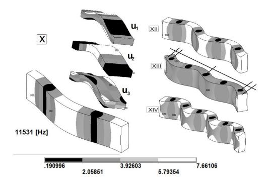
Figure 17: Three configuration modes on the dispersion curve d (see Figs.9 and 14), bending mode around the  $x_3$  axis. Configurations computed with the Method 2. Perceive that in mode XIII auxiliary lines indicate that in this case the wave enters 2.25 times in L=0.0628m, that is p=2.25.
