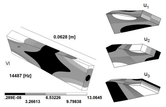
*Figure 13:* Mode associated with the point ck depicted in Fig.12, computed with Method 2. In the detail the displacement is presented. This modal configuration also corresponds to the point identified as (V) in the Fig.15. (In this case, p=0.5 is the number of the length wave that enters in the stem portion investigated, that has a length of L=0.0628m).
