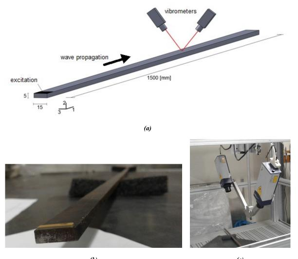
(b) (c) Figure 22: Experimental layout, (a) General scheme where the position of the laser vibrometer is fixed to measure a wave that propagates in the bar b) The ceramic pzt stuck in the specimen and c) The Polytec laser vibrometers.
