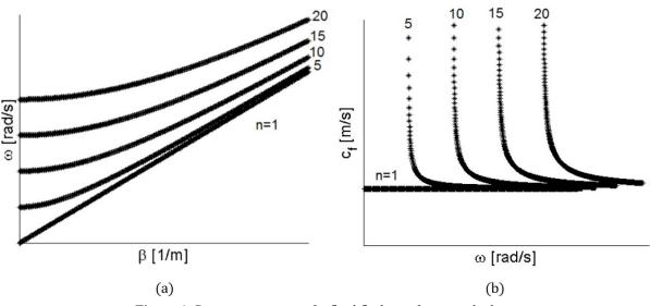
Figure 4: Dispersion curves of a fluid flysheet of unitary thickness
