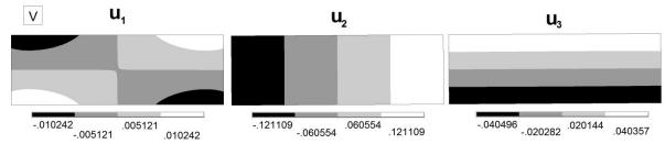
Figure 14: Mode linked to the point ck, depicted from Fig. 11, was computed using the Method 1 considering R = 50[m] and  $C_{order} = 2500$ . Then  $\lambda = 2\pi R/C_{order} = 0.1256m$ , and  $k = 2\pi/\lambda = 50$  m. The modal displacement  $u_2$ , according to the results obtained with the others methods, is the highest component. This modal configuration also corresponds with the point identified as (VI) in the Fig.15.
