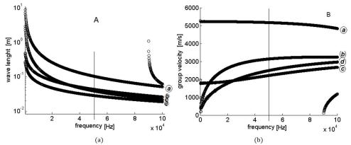
(a) (b) **Figure 10:** Dispersion curves (a) in terms of wave length vs frequency. (b) of group velocity vs frequency.
