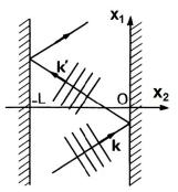
*Figure 3:* Guided waves propagation in a flysheet of fluid with thickness L, and with boundaries perfectly reflexive. Royer & Dieulesaint (1996).
