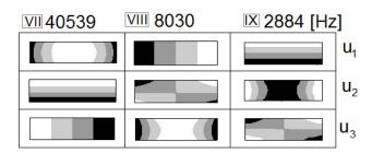
Figure 19: Displacement fields obtained with the Method 1 adopting R = 50 and  $C_{order} = 2,500$ . (equivalent to  $k=50 \text{ m}^{-1}$ ).
