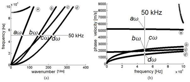
*Figure 9:* Dispersion curve (a) in terms of frequency vs wave number.(b) in terms of the phase velocity vs frequency. The displacement fields associated with the modes in the points  $(a\omega, b\omega, c\omega, d\omega)$  were presented in Fig. 11.
