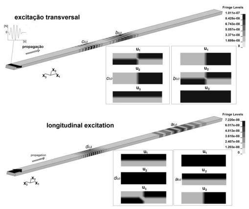
*Figure 20:* The numerical analysis of the excitation tone burst of 50KHz and five cycles over a metallic rectangular stem. The black arrow indicates the direction and region where the force was applied. The transversal views show displacement and they are done in the time when the wave passes through the transversal section of the stem. The images were extracted in the simulation in the time instant t = 0.275 [ms].
