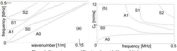
Figure 6: Dispersion curves of Titanium plate with 10 mm of thickness.
