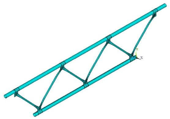
Figure 17: Truss numerical model.
