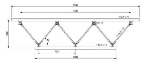
Figure 15: Plane truss geometry. Dimensions in milimeters.
