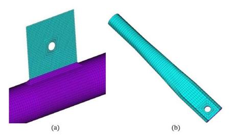
Figure 7: Representation of mesh. (a) Chord-plate-weld. (b) Stiffened-end diagonal.
