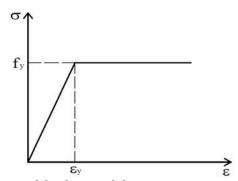
Figure 6: Schematic representation of the diagram bilinear stress-strain relationship used in the analyses
