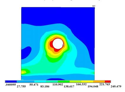
Figure 14: von Mises stress distribution (MPa) of the connecting plate for the load of 30 kN.
