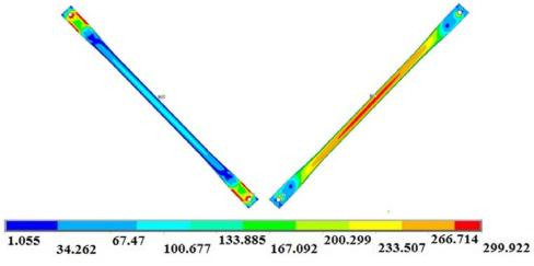
**Figure 22:** von Mises stress distribution (MPa) in the diagonal under compression for the load of 64 kN. View of the region under tension of the diagonal (left) and view of the region under compression of the diagonal (right).
