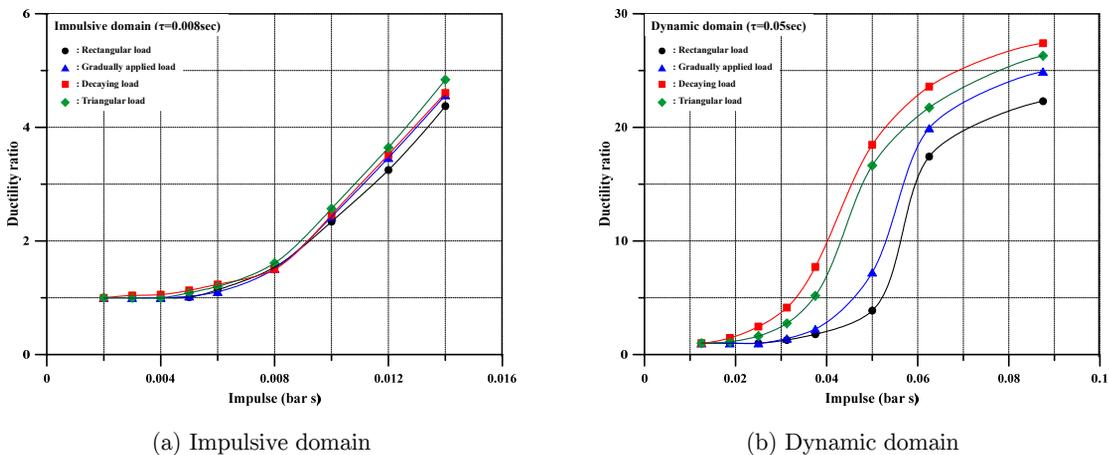
Figure 9: The dependency of the ductility ratio with increasing impulse for different loading pulse shapes.
