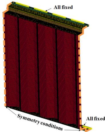
**Figure 2:** Nonlinear finite element model together with the applied boundary conditions.
