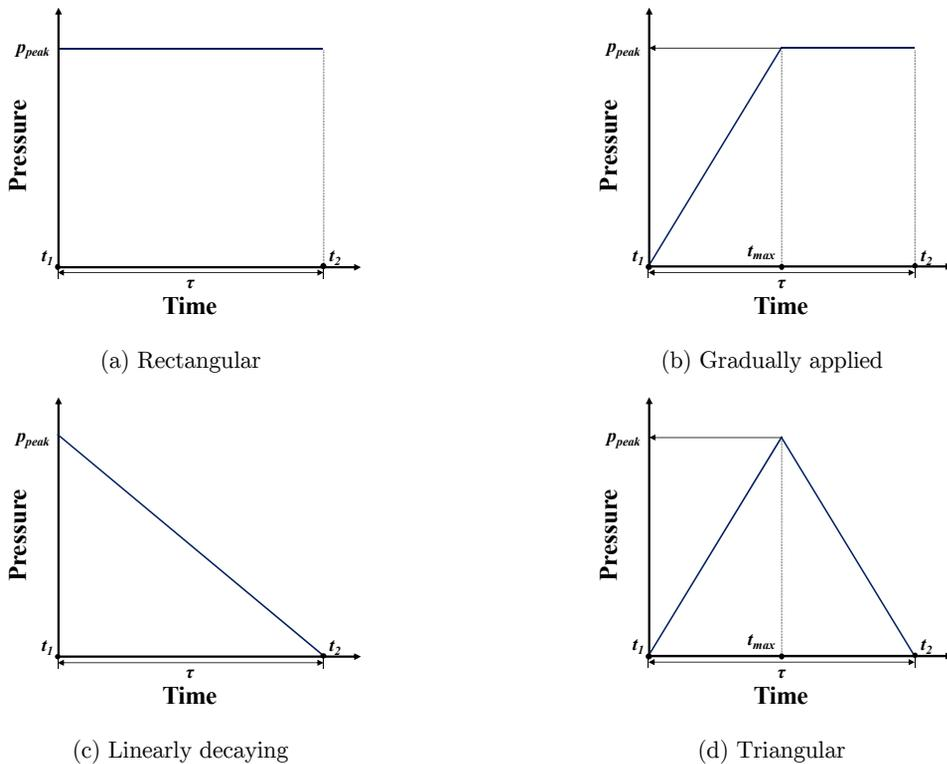
Figure 4: Common pulse loading shapes.
