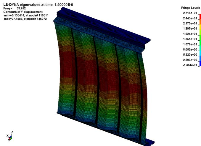
Figure 6: Resultant displacements for the modal analysis at 33.752Hz.
