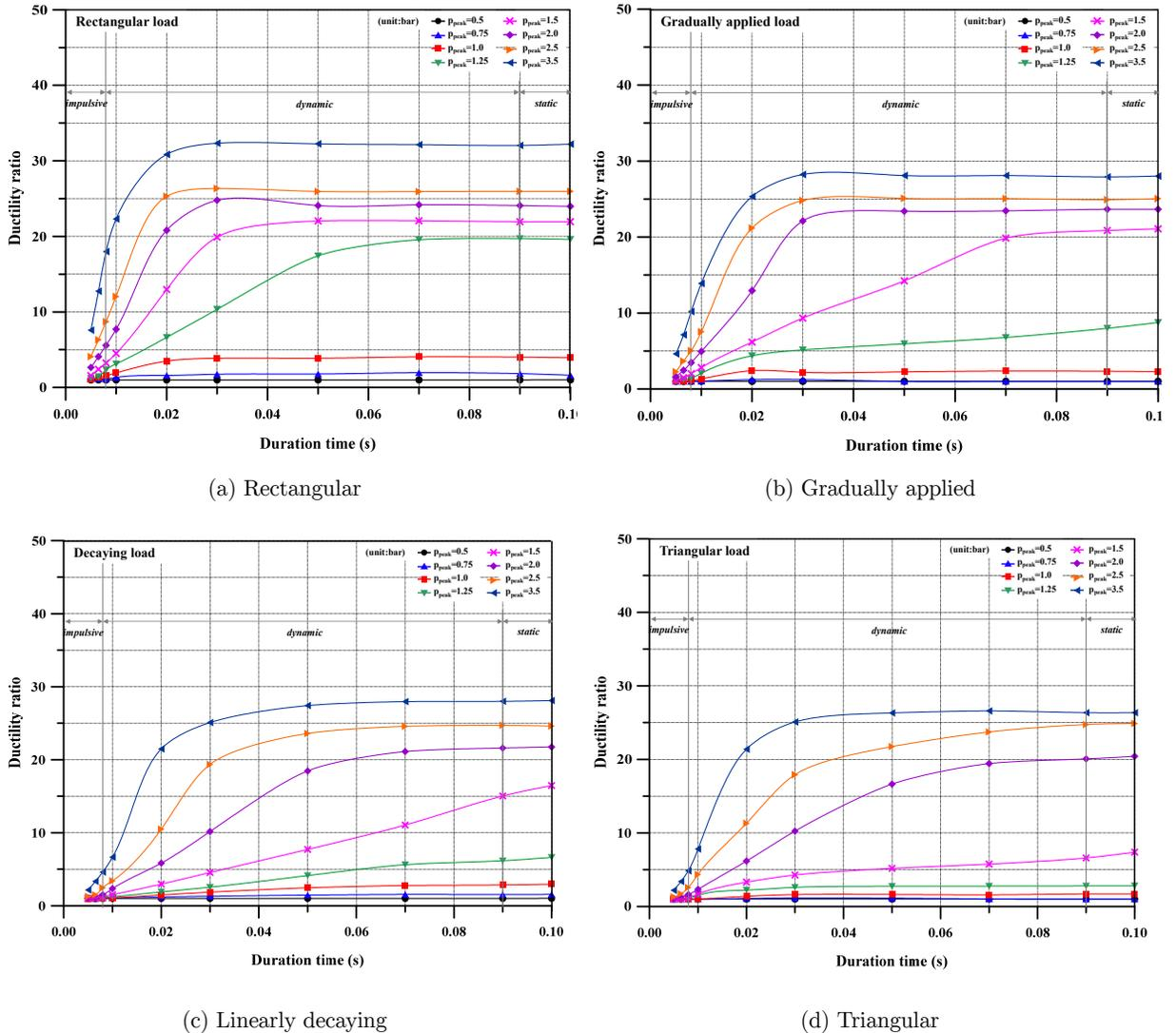
**Figure 7:** Ductility ratio as a function of duration time for several types of pressure-time histories with different peak pressures: (a) rectangular, (b) gradually applied, (c) linearly decaying, and (d) triangular.
