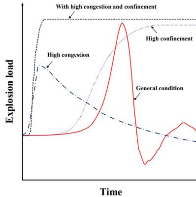
Figure 3: Explosion load profiles according to the congestion and/or confinement of structures (Kim 2016).
