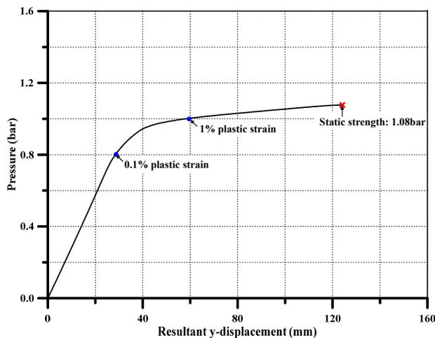
Figure 5: Result of static push-over analysis of a blast wall.
