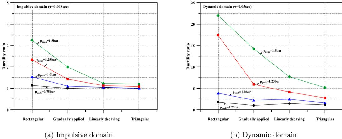
Figure 8: Comparison of the change in ductility ratio for various pulse shapes.
