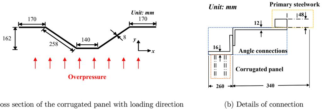
Figure 1: Main dimensions of blast wall in the present study (HSE, 2003).
