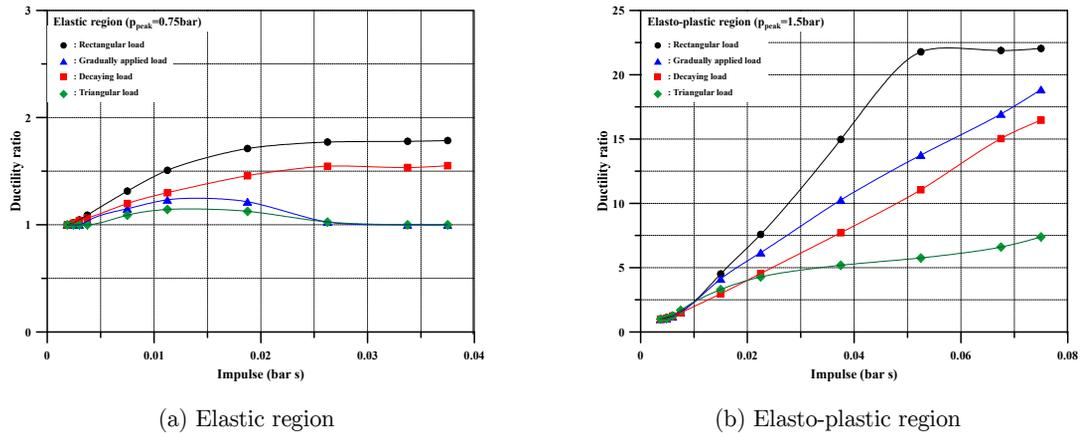
**Figure 10:** Ductility ratio versus impulse curves for different loading pulse shapes at a specific peak pressure.
