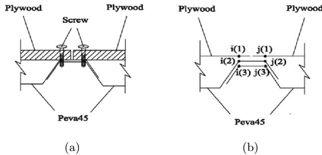
Figure 8 Detail A: (a) Constructional model (b) Analytical model
