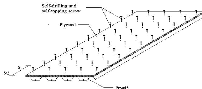
Figure 2 Profiled steel sheet dry board system.
