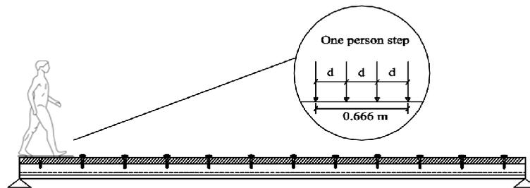
Figure 5 Person walking on the PSSDBC floor panel.
