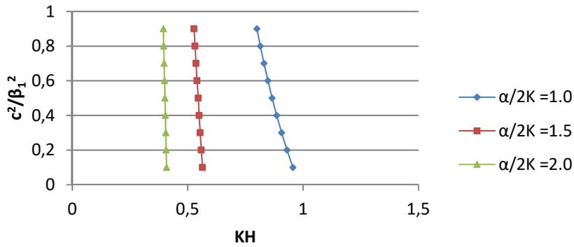
**Figure 2:** Variation of dimensionless phase velocity  $(c/\beta_1)^2$  against dimensionless wave number KH demonstrating the influence of non-homogeneity associated with upper crustal layer for  $n/K = 1.0$ ,  $H_2/H_1 = 1.0$ .
