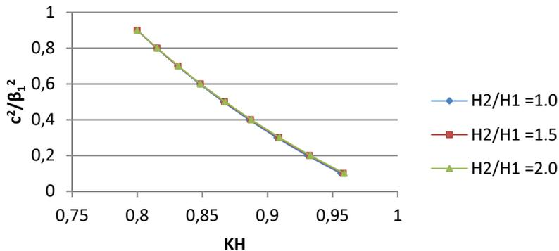
**Figure 4:** Variation of dimensionless phase velocity  $(c/\beta_1)^2$  against dimensionless wave number KH demonstrating the influence of thickness ratio  $H_2/H_1$  for  $\alpha/2K = 1.0$ ,  $n/K = 1.0$ .
