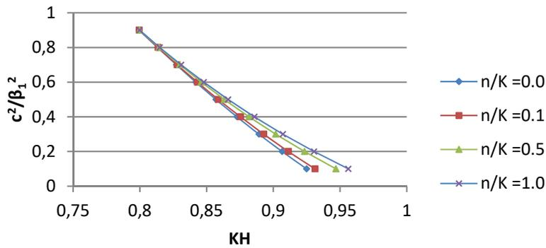
**Figure 3:** Variation of dimensionless phase velocity  $(c/\beta_1)^2$  against dimensionless wave number KH demonstrating the influence of non-homogeneity associated with intermediate crustal layer for  $\alpha/2K = 1.0$ ,  $H_2/H_1 = 1.0$ .
