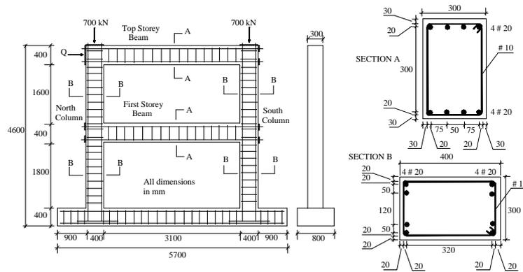
Figure 5: Geometry and reinforced details of the frame
