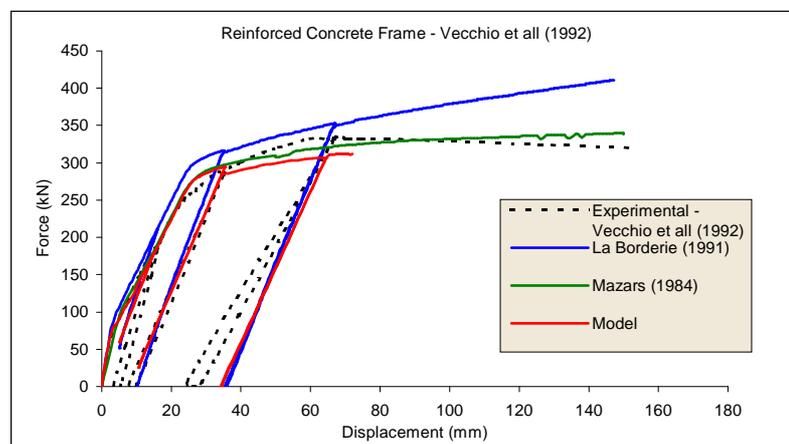
Figure 6: One-dimensional frame analysis: experimental and numerical results
