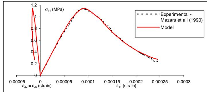
Figure 1: Simulation of the uniaxial tension test: experimental and numerical results.
