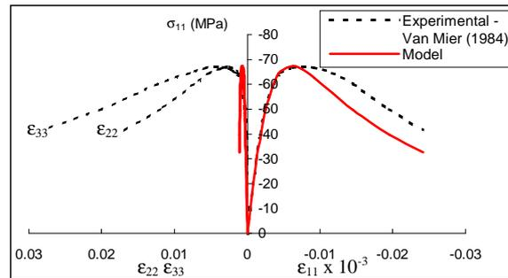
Figure 3: Simulation of triaxial compression test: experimental and numerical results.
