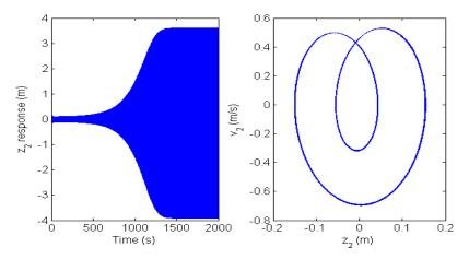
Fig. 3(b):  $z_2$ - waveform and phase plot ( $\omega = 5.1 \text{ rad/s}$ ).
