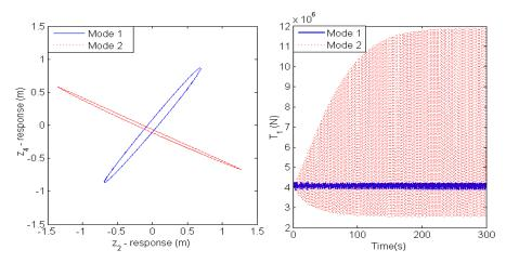
Fig. 7(b): Modal Lissajous plots and modal tension  $T_1$  waveforms.
