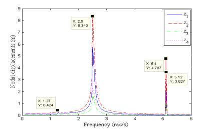
Fig. 3(a): Typical FDR for general forcing function.
