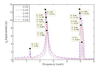
Fig. 4: Effect of peak sinusoidal forces on FDR.
