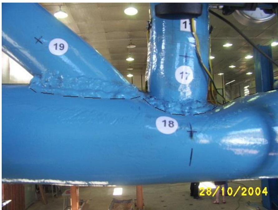
Figure 6 Failure Mode A: plastic failure of the chord face at EXPERIMENT II.
