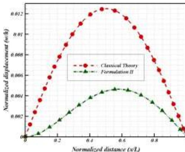
**Figure 6:** Normalized displacement of a simply-supported beam according to the classical theory and formulation II with  $L=20h$ ,  $b=2h$ ,  $h=10g$  and  $g=0.02$  nm.
