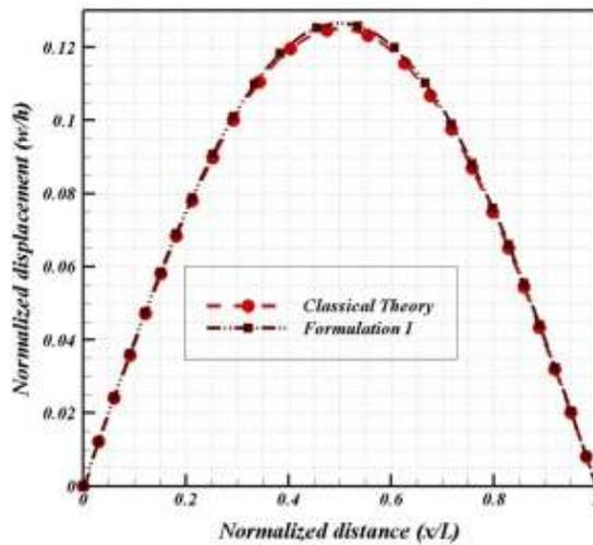
**Figure 4:** Normalized displacement of a simply-supported beam according to the classical theory and formulation I with  $L=20h$ ,  $b=2h$ ,  $h=g$  and  $g=0.02$  nm.
