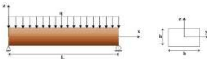
Figure 1: The simply-supported nano-beam subjected to a constant distributed load.
