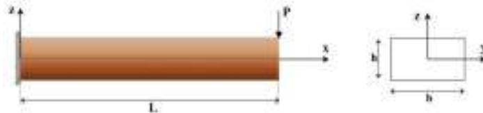
**Figure 2:** The cantilever nano-beam subjected to a tip-point load.
