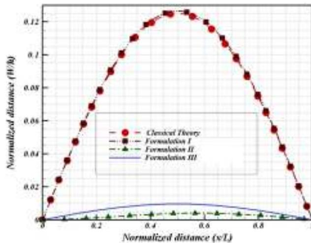
**Figure 8:** Normalized displacement of a simply-supported beam according to different theories with  $L=20h$ ,  $b=2h$ ,  $h=g$  and  $g=0.02$  nm.
