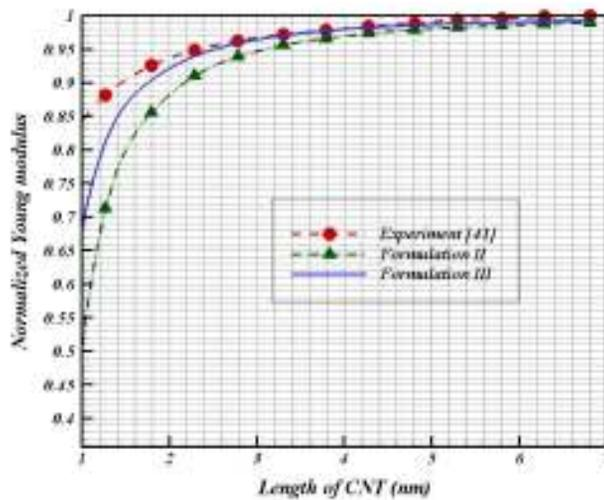
**Figure 13:** Normalized Young's modulus of CNT, based on strain gradient elasticity theories and experimental predictions.
