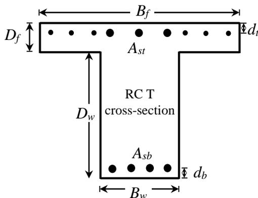
Figure 7: T cross-section.
