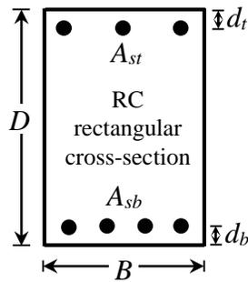
Figure 2: Rectangular cross-section.
