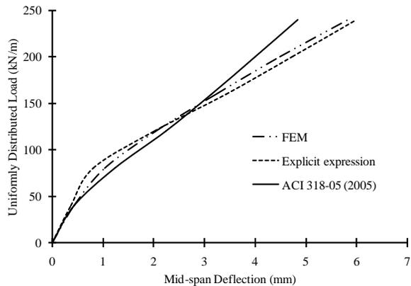
Figure 8: Comparison of mid-span deflections of beam VB11.
