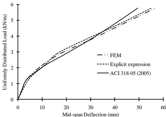
Figure 11: Comparison of mid-span deflections of beam VB14.
