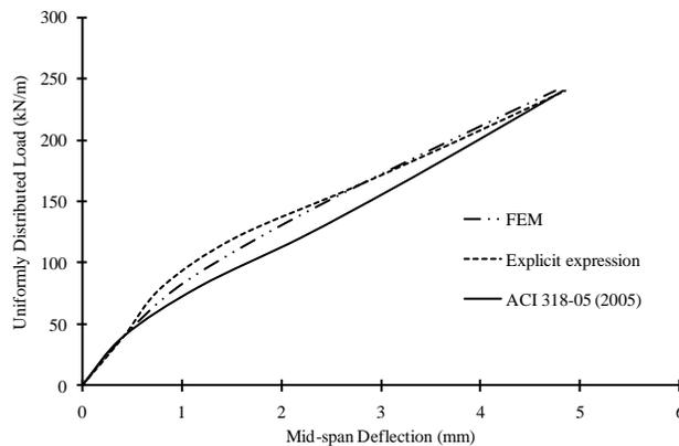
Figure 9: Comparison of mid-span deflections of beam VB12.
