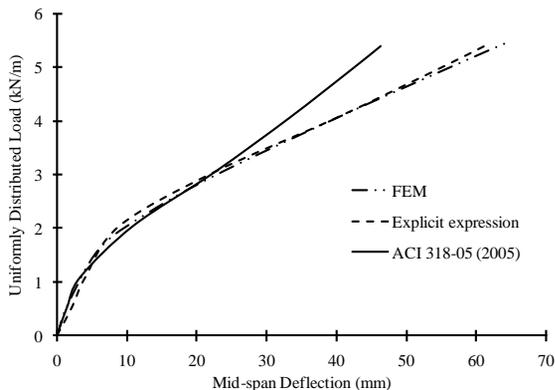
Figure 10: Comparison of mid-span deflections of beam VB13.
