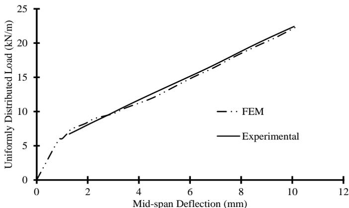
Figure 3: Comparison of mid-span deflections of beam VB.
