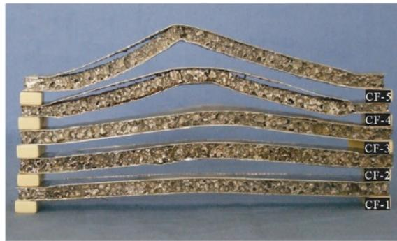
Figure 3 Experimental results of impact failure modes with respect to load intensity (Wang, et al., 2011).
